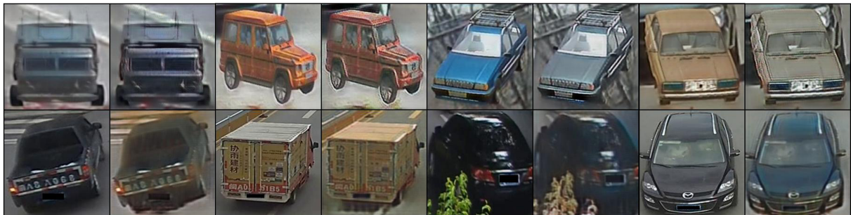
Fig. 1. Results on mapping synthetic images to real-world styles and vice versa. Each pair displays the source and target, with the origin image on the left and the generated image on the right. The top row showcases synthetic images from the Vehicle-X dataset, while the bottom row presents real images from the VeRI dataset.
